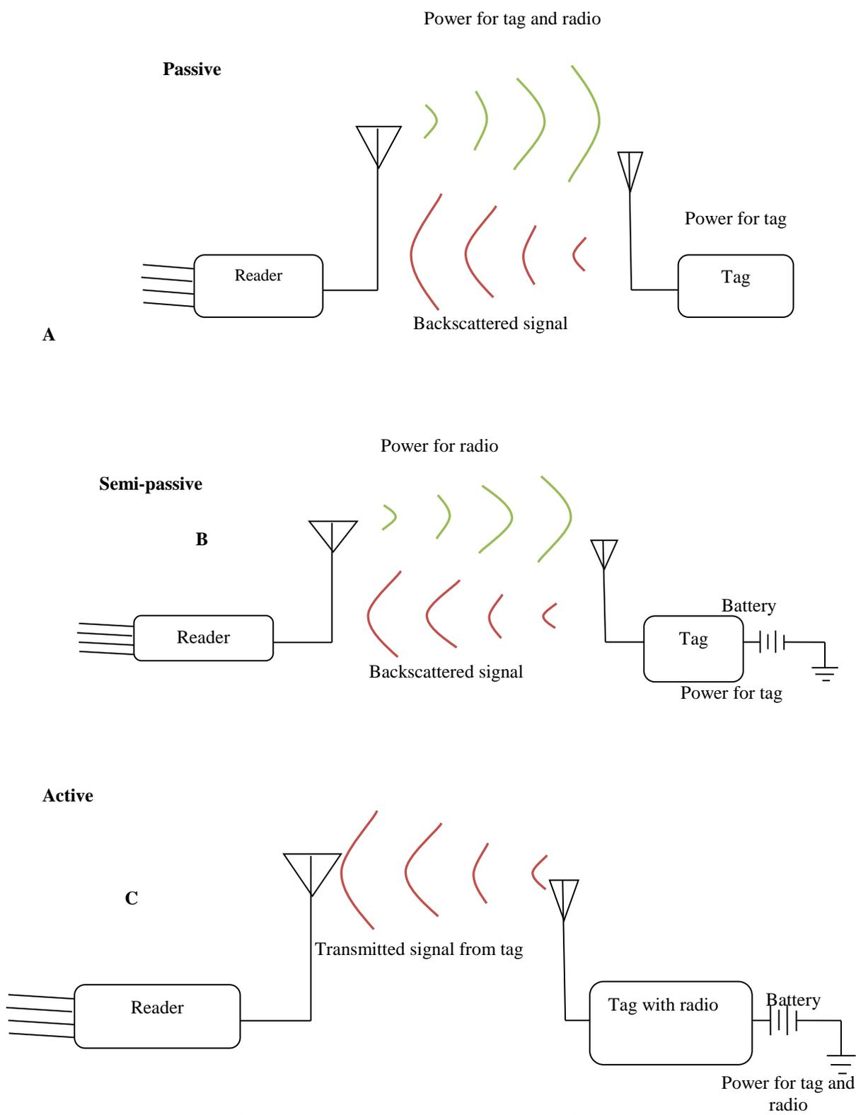
Figure 1: Function of (A) passive, (B) semi-passive and (C) active RFID tags.
